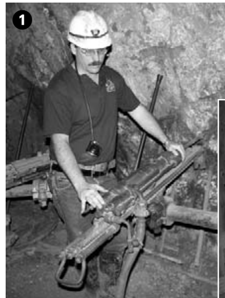
① A miner would use the drill, above, ② to make holes in the rock, top right. ③ A stick of dynamite would go into each hole before being wired for blasting, bottom right.
